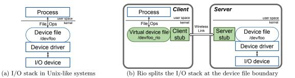
Figure 1: Rio splits the I/O stack at the device file boundary. The process that remotely uses the I/O device resides in the client system and interacts with a virtual device file. The actual device file, device driver, and I/O device all reside in the server system. Rio forwards file operations between the client and server. The wireless link can either be through an AP or a device-to-device connection.
