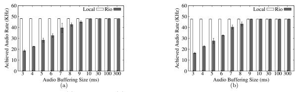
Figure 6: Performance of (a) speaker and (b) microphone. The X axis shows the buffering size in the HAL. The larger the buffer size, the smoother the playback/capture, but the larger the audio latency. The Y axis shows the achieved audio rate.
