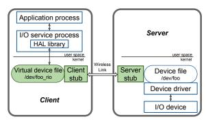
Figure 4: Rio's architecture inside an Android system. Rio forwards to the server the file operations issued by the I/O service process through HAL. Rio supports unmodified applications but requires small changes to the class-specific I/O service process and/or HAL.
