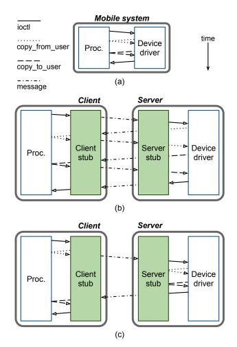
Figure 3: Typical execution of an ioctl file operation for (a) a local I/O device, (b) a remote I/O device with unoptimized Rio ( $\S4.2$ ), and (c) a remote I/O device with optimized Rio ( $\S5.1$ ). As the figure shows, optimized Rio reduces the number of round trips from 3 to 1. The reduction can be even more significant if the file operation requires more copy memory operations.
