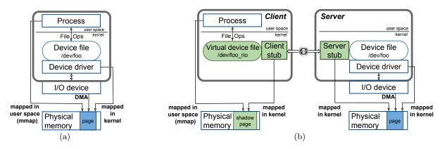
Figure 2: (a) Memory map for a local I/O device. (b) Cross-system memory map in Rio.
