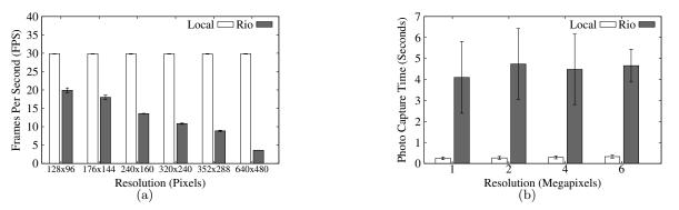
Figure 7: Performance of a real-time streaming camera preview (a) and photo capture (b) with a 21.9 Mbps wireless LAN connection between the client and server. Future wireless standards with higher throughput will improve performance without requiring changes to Rio.
