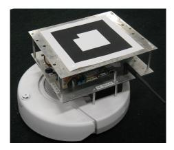
Figure 3. Our mobile robot: Roomba with top-mounted decal.
